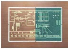
Circuit board without solder-resist lacquer (left), with solder-resist lacquer (right)
