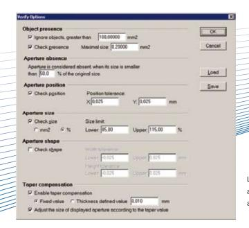
LPKF StencilCheck offers numerous individually adjustable parameters e.g. for aperture size, aperture shape and position.
